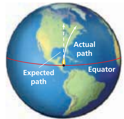
■ Figure 8-17 An observer on Earth sees the Coriolis “force” cause a projectile fired due north to deflect to the right of the intended target.
