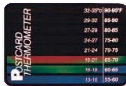
■ Figure 12-4 Thermometers use a change in physical properties to measure temperature. A liquid-crystal thermometer changes color with a temperature change.
