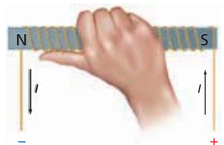
■ Figure 24-12 The second right-hand rule can be used to determine the polarity of an electromagnet.
