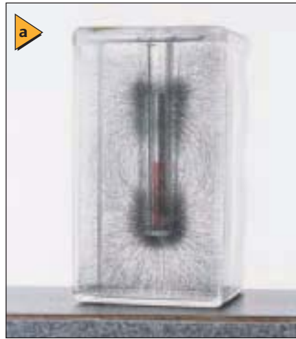
■ Figure 24-4 The magnetic field of a bar magnet shows up clearly in three dimensions when the magnet is suspended in glycerol with iron filings (a) . It is, however, easier to set up a magnet on a sheet of paper covered with iron filings to see the pattern in two dimensions (b) .
