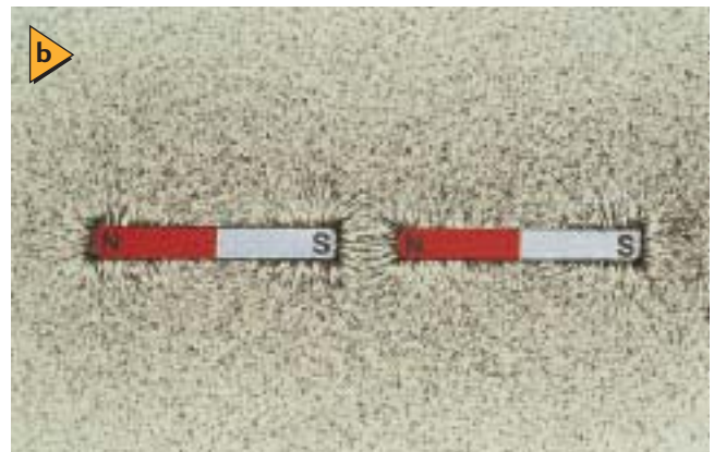
■ Figure 24-6 The magnetic field lines indicated by iron filings on paper clearly show that like poles repel (a) and unlike poles attract (b) . The iron filings do not form continuous lines between like poles. Between a north and a south pole, however, the iron filings show that field lines run directly between the two magnets.
